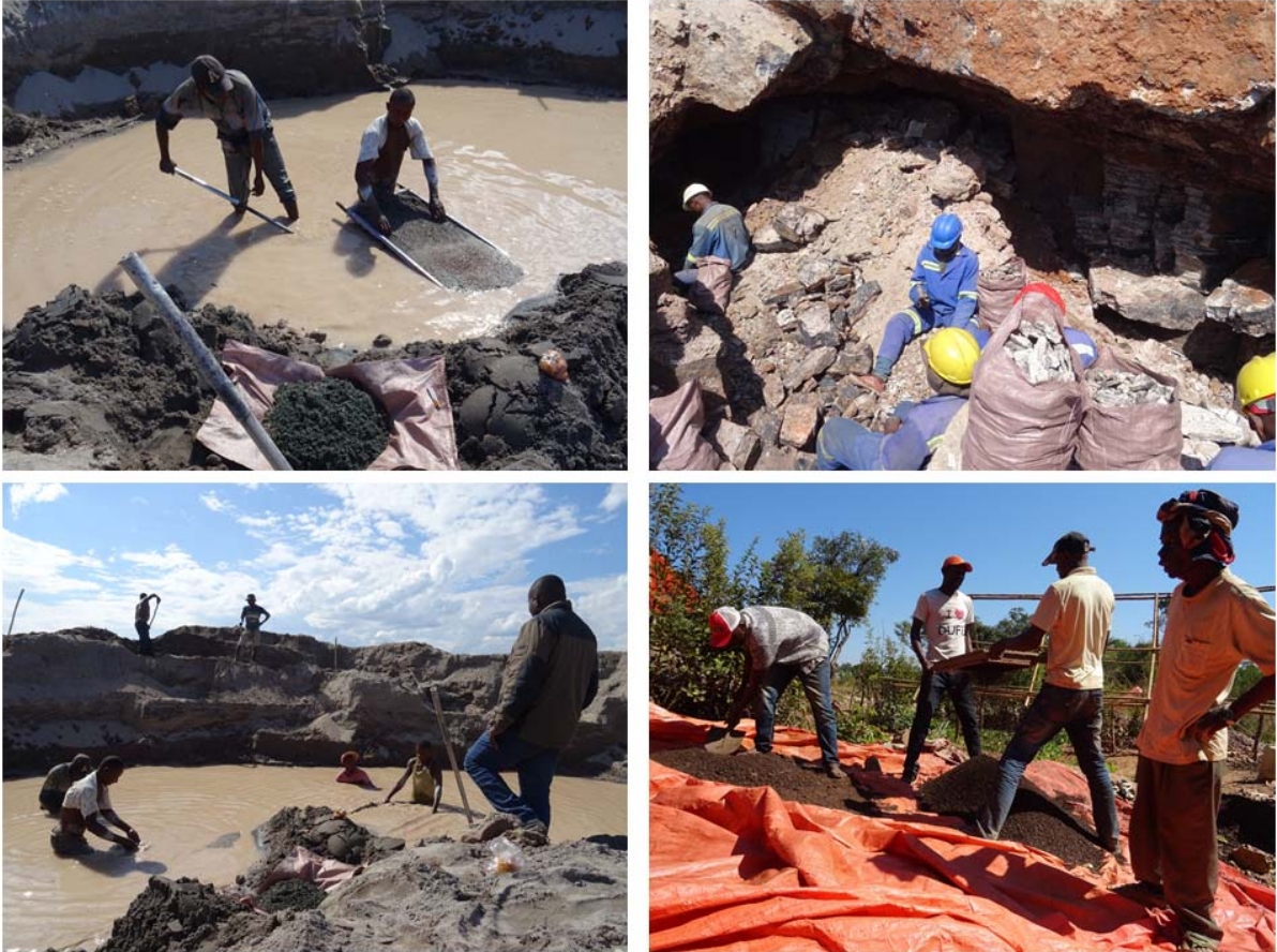
Figure 13 Processing techniques for copper and cobalt in Congolese artisanal mining. Washing and crushing processes as well as the sieving of previously washed ores can be seen.
