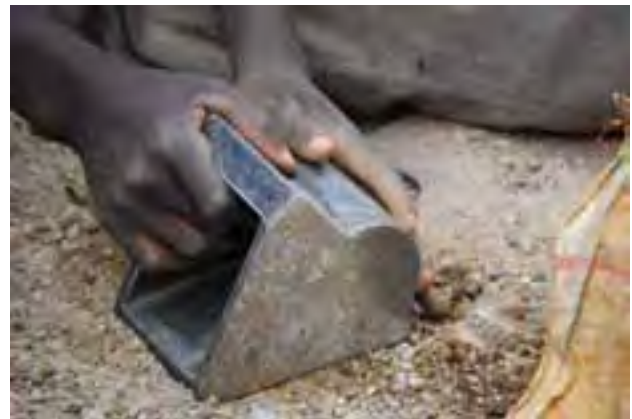
Gold and mercury 'amalgum' (Top); Old machine piece being used as a cassiterite rock crusher (Bottom).
